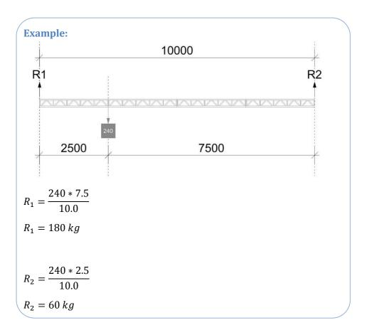
For more than one point, the above formula can be used for each point load and the values for  $R_1$  and  $R_2$  can be summed to give the total resultants.
