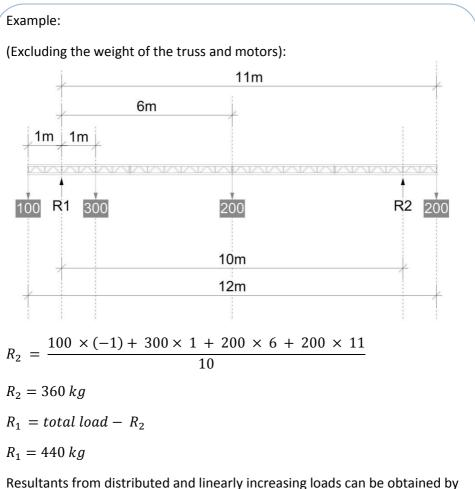
Resultants from distributed and linearly increasing loads can be obtained by applying the total load as a point load through the centre of gravity of the element.
