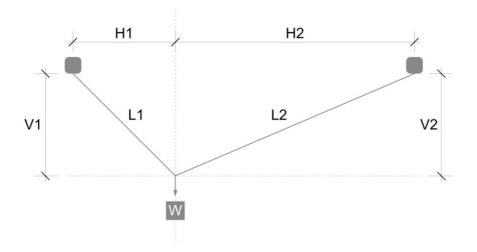
Calculating the length of a bridle leg is performed using Pythagoras' theorem:
